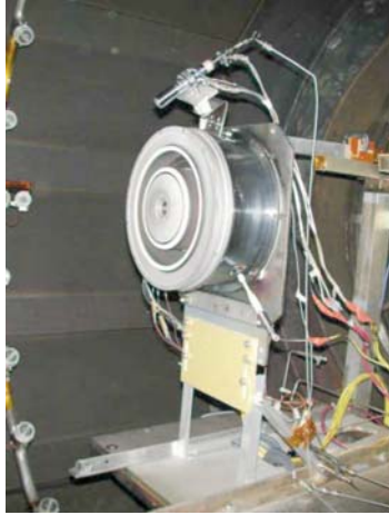
Figure 1. T-220HT mounted in vacuum chamber #3 at AFRL.
