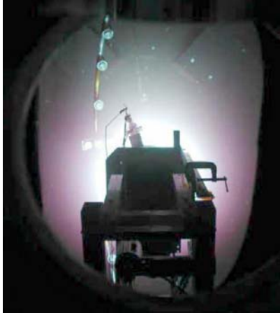
Figure 6. View from behind T-220HT showing probe rake sweeping through the plume.
