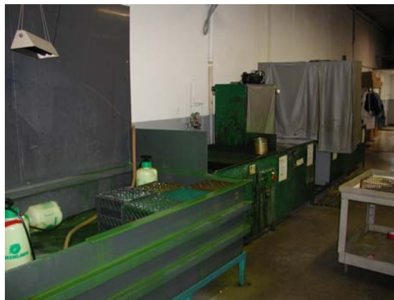
Figure 4, Vendor Fluorescent Penetrant Line
