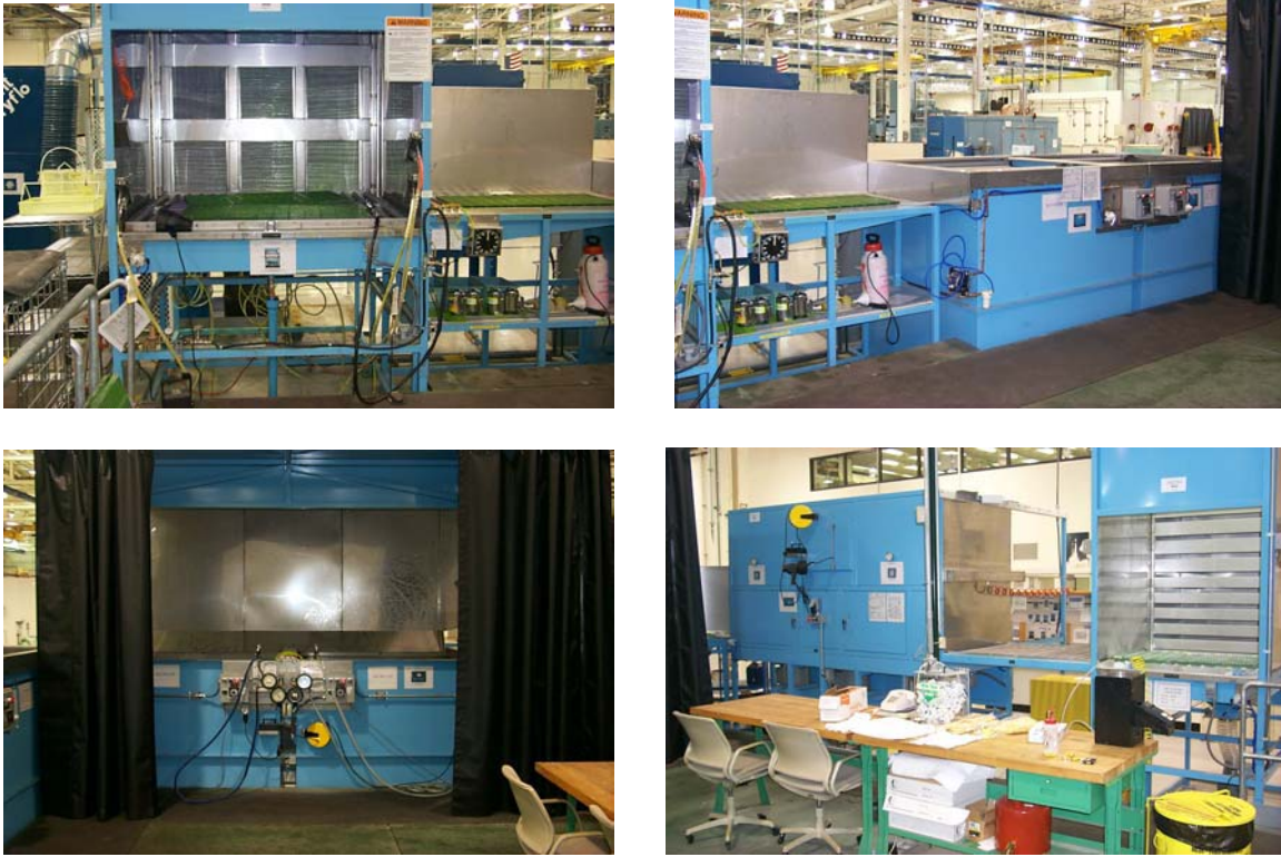
Figure 3, P&W Space Propulsion Fluorescent Penetrant Line
